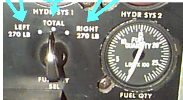
Figure 6-15 Fuel Quantity Indicating System
