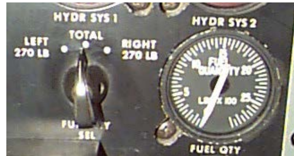
Figure 6-14 Fuel Quantity Selector
