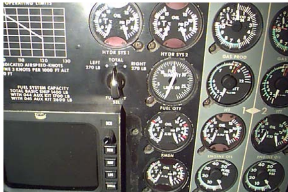
Figure 6-16 Fuel Gauges Selector Switch
