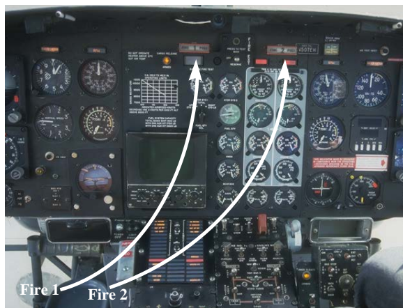
Figure 6-11 Fire Pull Handles
