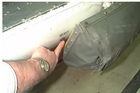
Figure 6-6c Fuel Sump Drain System
