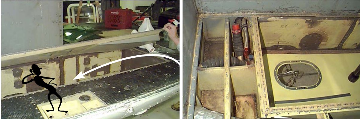
Figure 6-2 Lower Fuel Cell Location
